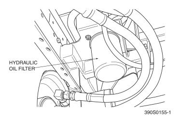
Figure 7-3. Hydraulic Oil Filter
